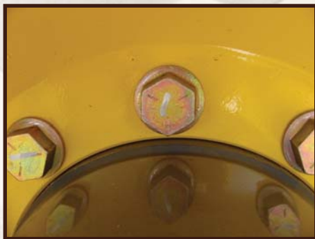
Grade 5 bolt head identification
