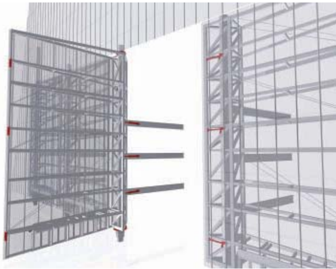
Turning cylinders and upper and lower pivot bearings move the large doors, and lock bars secure them during high winds or other extreme weather events, above left . Each door pivots about a fixed building column, above right , located approximately 5 ft from the north edge of the door.
